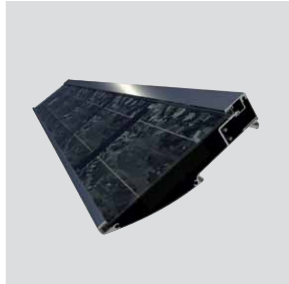
Photovoltaic modules 185 x 1200 mm Polycrystalline cells (27 Wc) or monocrystalline cells (28 Wc)
